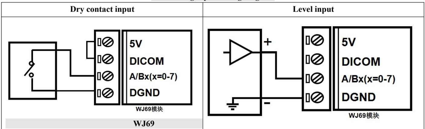
**Encoder signal input wiring diagram**
