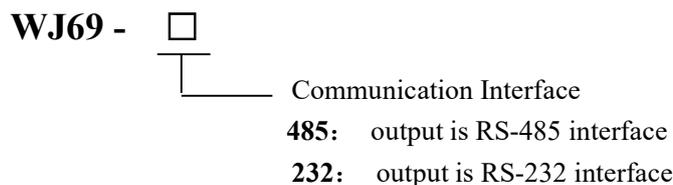
Sample 1: part No.:WJ69-232 means output is RS-232 interface
