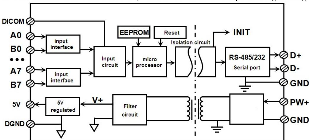
Figure 2: WJ69 Block Diagram
