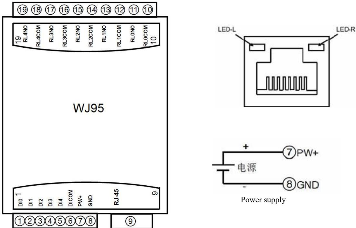
Figure 5 WJ95-RJ45 Wiring Diagram
