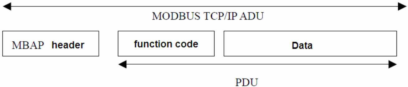
**Figure 6: MODBUS request/response over TCP/IP**
